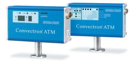
The Convectron ATM module is available in both analog output or RS-485 interface versions. The Convectron heat loss sensor provides vacuum pressure measurement over seven decades from  $1 \times 10^{-4}$  Torr to atmosphere. The diaphragm sensor technology measures the differential pressure between the inside of the vacuum space and the outside environment and activates a setpoint relay when a defined differential pressure is achieved.
